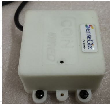
Use Screws or Cable ties on flange
